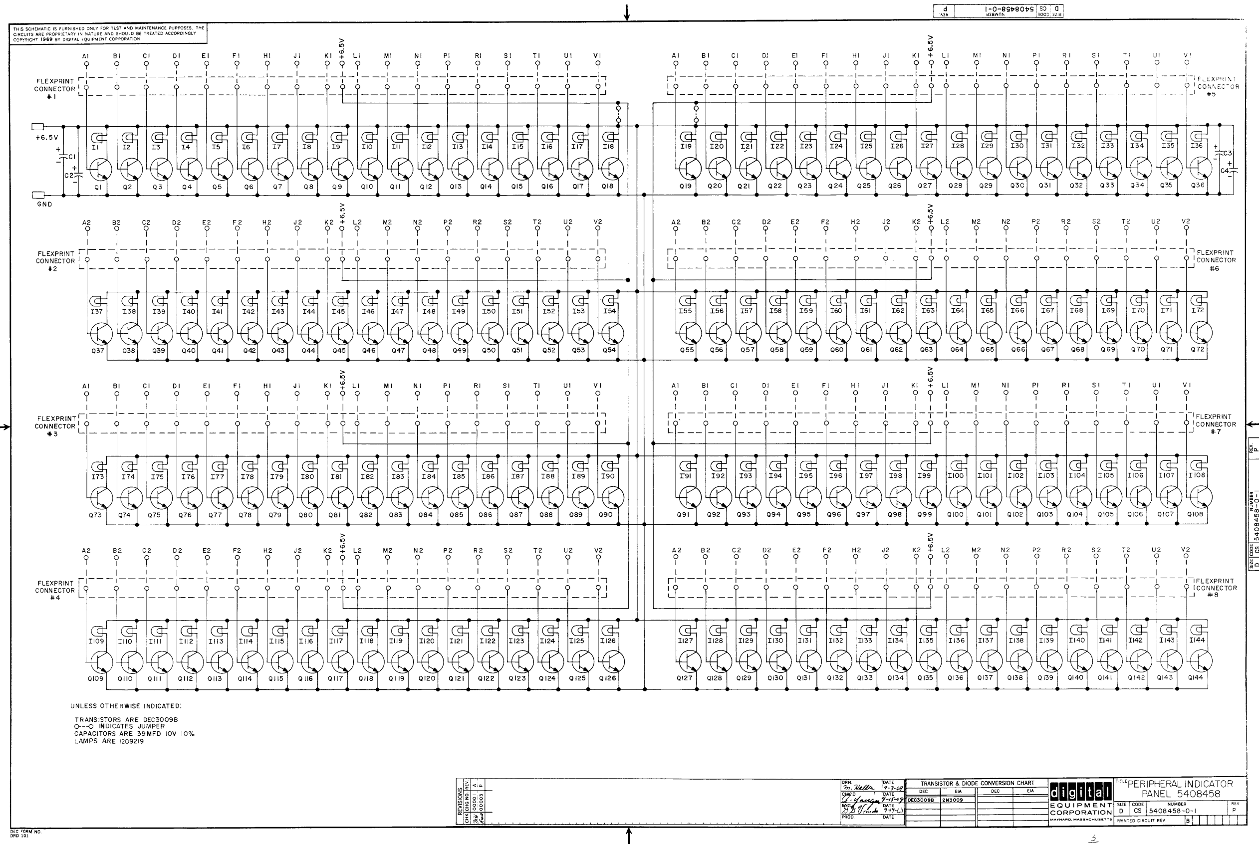
Figure II-42 Register Indicator Panel Circuit Schematic Diagram
