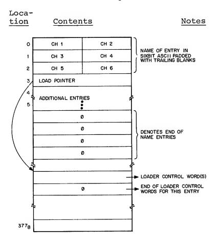
The Load Pointer is a number between 0 and 377<sub>8</sub> which points (relative to the beginning of the block) to an array of Loader Control Words. The Loader Control Words have the following information:
