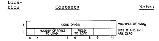
The core origin must be a multiple of  $400_8$ . The Core Segment Control Doublewords are sorted within the header block in order of decreasing field and increasing origin within the same field. There can be no more than  $32_{10}$  Core Segment Control Doublewords in any Core Control Block.
