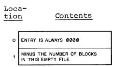
A <u>tentative file</u> entry appears as a permanent file entry with a length of zero. It is always immediately followed by an empty file entry. When the tentative file is entered in a directory, location 3 in the segment header becomes a pointer to this entry. The CLOSE function inserts the length word of the tentative file entry, making it a permanent file, and adjusts the length of the following empty file entry (deleting that entry if the length becomes zero).
