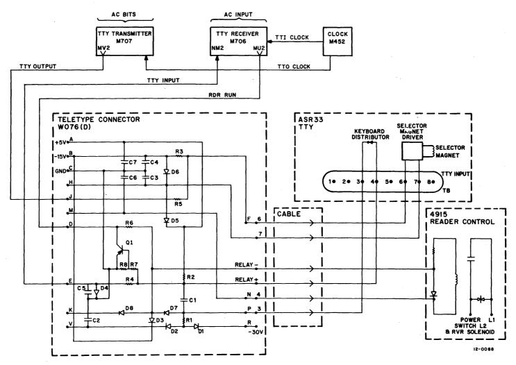
Figure 5-1 Teletype Connections
