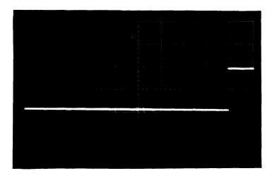
Figure 3-5 Teletype Clock (Sweep at .5 ms)
