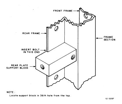
Figure 4-7 Rear Plate Assembly of TU56
