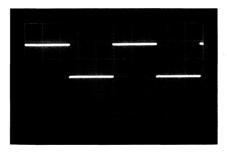
Figure 3-19 25 ms Oscillator Adjustment
