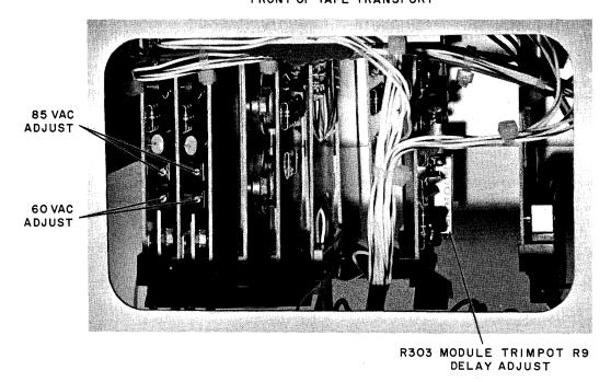
Figure 3-15 TU55 Stop Delay Adjustment
