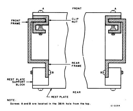
Figure 4-8 Top View of TU56 Rest Plate Assembly
