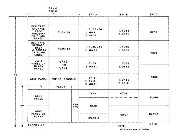
Figure 1-3 PDP-12 Expanded Equipment Layout (see Drawing PDP12-0-2)
