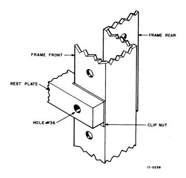
Figure 4-6 Front Assembly of TU56
