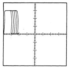
NOTE: A RAGGED TRAILING EDGE IS CAUSED BY TAPE BOUNCE
