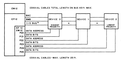
\* If the priority interrupt system is used in the KF12B this cable is connected separately from each device.
