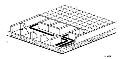
Figure 1-2 Raceway Flooring
