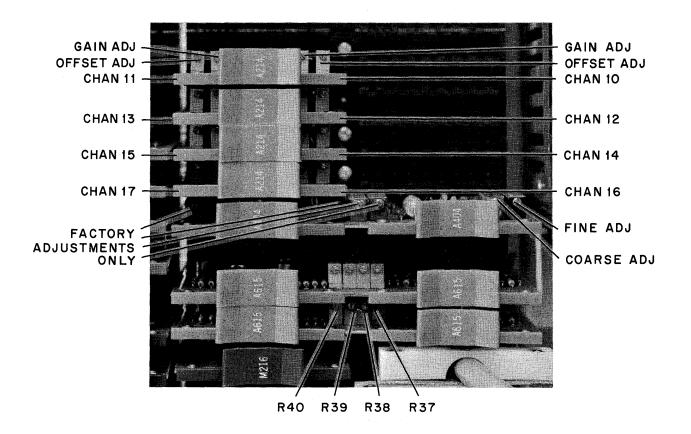
Figure 3-21 Sample and Hold Adjustments
