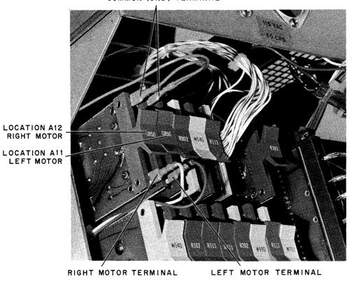
Figure 3-14 TU55 Torque Adjustment Tabs
