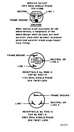
Figure 1-6 Hubbell Wall Receptacle Connector Diagram
