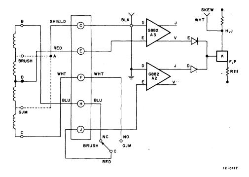
Figure 3-16 Skew Checker Schematic Diagram
