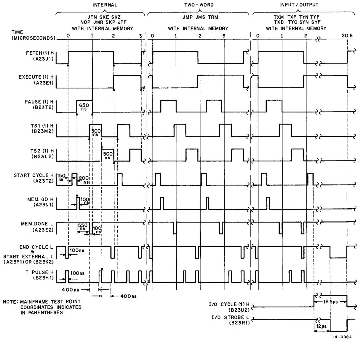
Figure 3-7 Control Logic Timing Diagram
