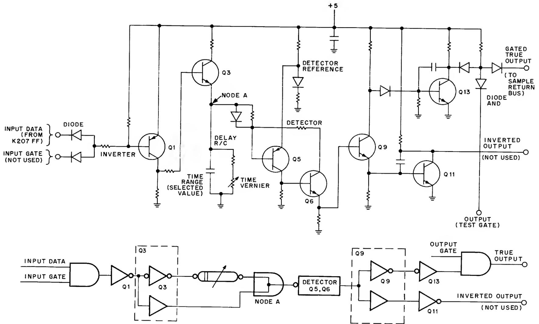
Figure 3-20 Timer Module, Time Delay Circuit, Simplified Schematic Diagram, and Equivalent Logic Diagram
