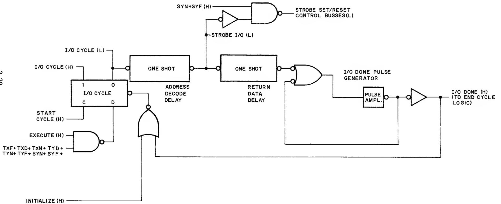
Figure 3-11 I/O Cycle Control, Simplified Logic Diagram
