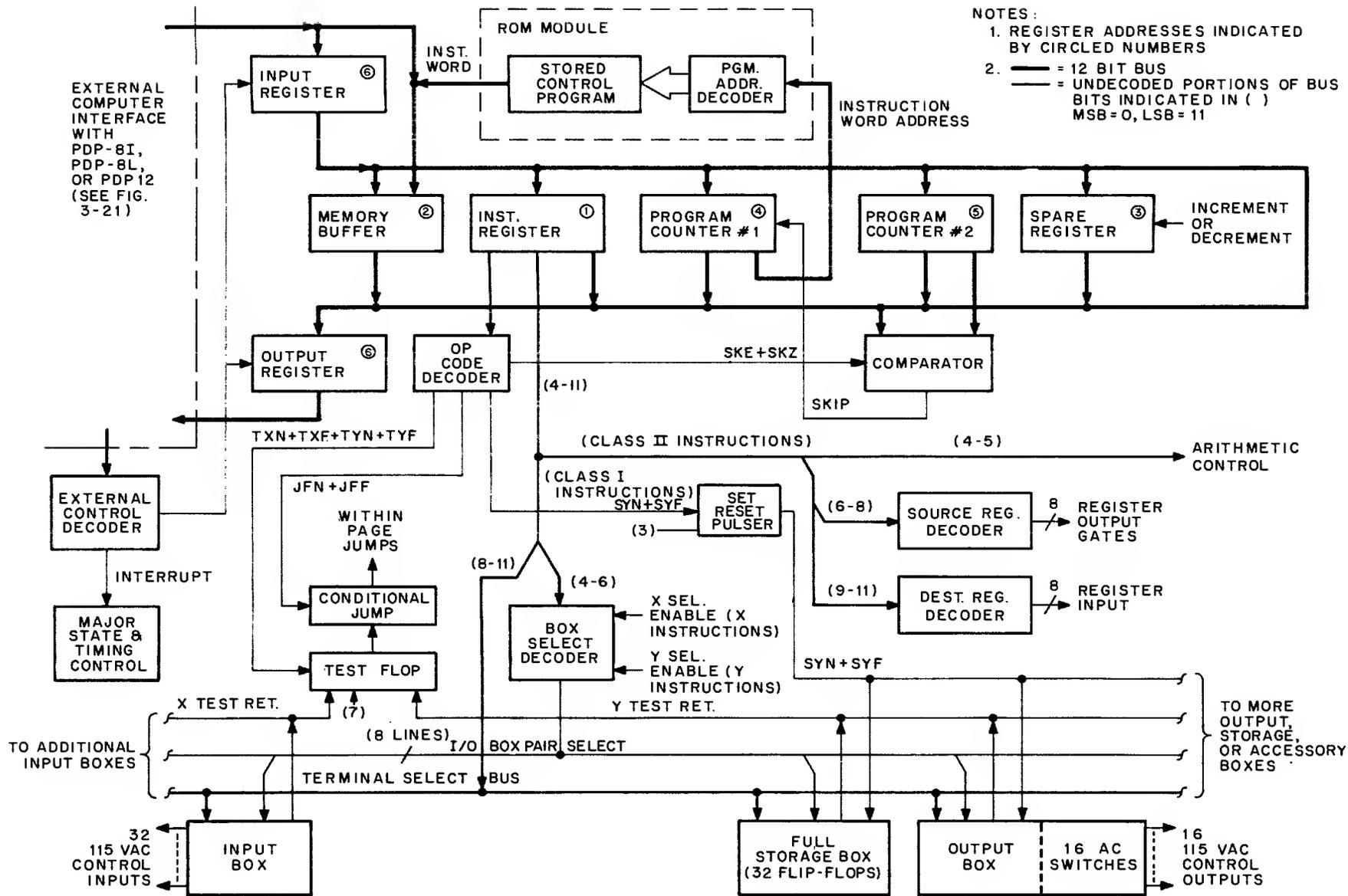
Figure 3-2 PDP-14 Controller, Detailed Block Diagram
