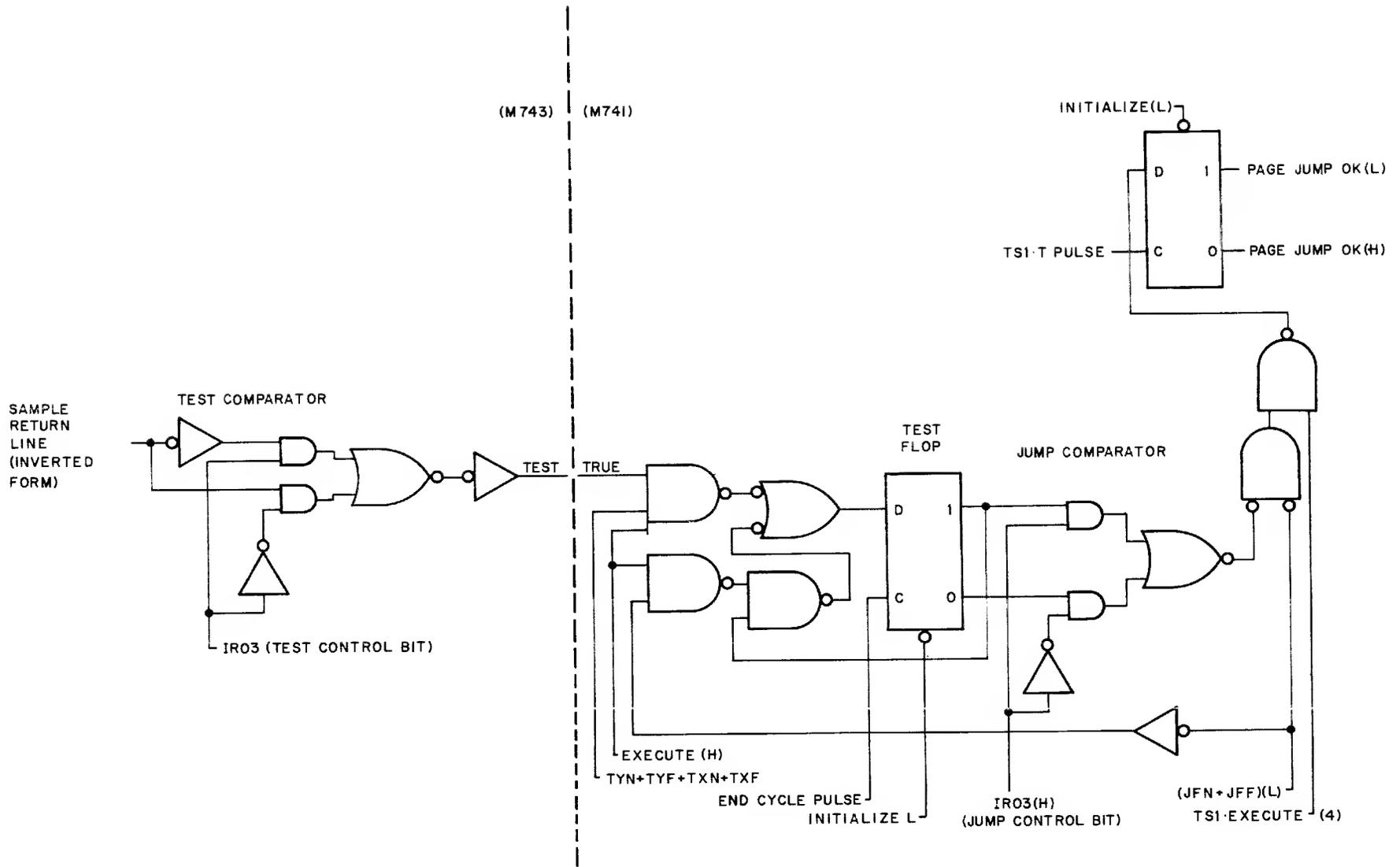
Figure 3-5 Test Flop and Associated Circuits, Simplified Logic Diagram
