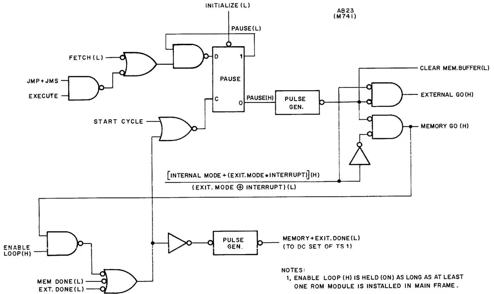
Figure 3-10 Pause Cycle Control, Simplified Logic Diagram
