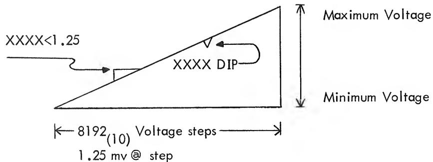
Case (a) is where the converted value 1374 was found, but before 1376 was found the converted value 1400 was reached. This infers that the voltage state which generates the converted value is less than 1.25 mv wide.
