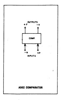
The A502 Comparator is a high speed difference amplifier which compares two input voltages and indicates which of the two is the more negative. The comparator has a resolution of 1 mv, and an input range of 0 to -10v. The maximum combined error due to a change in the common input voltage from 0 to -10v and a 20°C temperature change is 5 mv equivalent input offset. Two potentiometers allow adjustment of the zero set and common balance.
