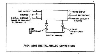
The A604 and A605 are two-bit digital-to-analog conversion modules for use with the A601 in forming high resolution, high accuracy converters. Inputs
