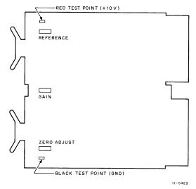
the polarity of the EDC connections to find the most negative switching point. Record the voltage. The difference between the voltages should be 19.9995V,  $\pm 2$  mV. Adjust the gain potentiometer and repeat these measurements until the difference is within the specified tolerance.
