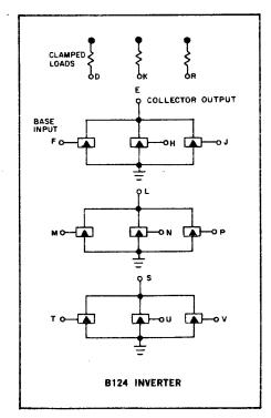
The B104 contains three standard 10-ma clamped loads and four transistor inverters, each with its base, emitter, and collector brought to connector pins.
