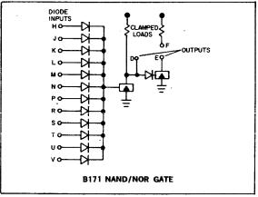
The B113, B115, B117, and B171 are positive NOR diode gates; they form NOR gates for ground inputs and NAND gates for —3 v inputs. The outputs of the diode gates drive inverters similar to the B105, for power amplification. The typical total transition time is 40 nsec for output fall and 60 nsec for output rise. (Because the rise and fall delays differ, these diode gates may shorten negative input pulses markedly; see below.)
