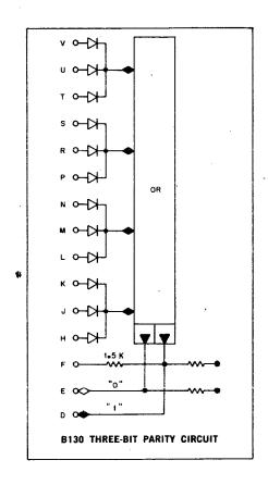
This special logic module has two levels of high speed logic and complementary outputs. It is designed to compute the parity (odd or even) of the contents of a flip-flop register with a minimum of time delay, but it can be used wherever there is a need for four 3-input negative diode AND gates feeding a 4-input OR gate.
