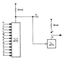
The B172 provides a 12-input 2 mA diode gate with 2 mA diode inverter permanently connected to the output of the first gate. It is often used for memory module selection on the PDP-10 memory bus.
