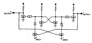
The B201 has nine built-in inverters for accomplishing such operations as set, clear, jam-transfer, shift, and complement without the need for additional gating. The B201 can also be used in counters. Logic diagrams for these operations are shown under "B Series Logic Configurations."
