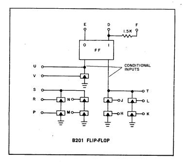
Some 10 mc operations require a greater variety of pulse inputs than the B200 can provide. For example read in from several sources, bi-directional shifting, and arithmetic operations all require the greater flexibility of the B201.
