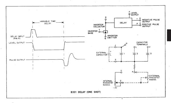
A delay (one shot) is a monostable multivibrator. When the input terminal is grounded, either through the inverter or externally, the level output switches from its normal ground level to -3 v for a predetermined, but adjustable, period of time; then it switches back to ground. Simultaneously with the final transition, a standard 40-nsec pulse is generated at the pulse output.
