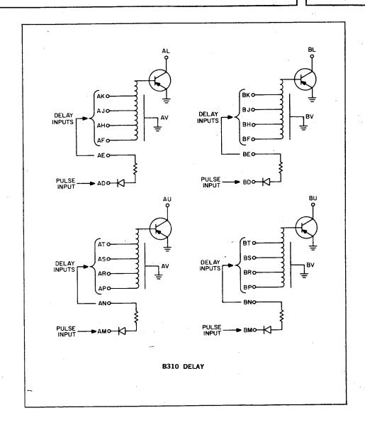
The B310 contains four delay lines, each producing maximum delay of 50 nsec in 12.5 nsec steps. The output of each line is connected to a transistor inverter whose emitter is grounded. The collector terminal is available for logical gating. The 15 nsec delay through the inverter must be added to the delay of the line.
