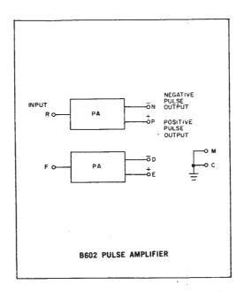
The B602 contains two pulse amplifiers which are used for power amplification, for standardizing pulses in amplitude and width, and for transforming a level change to a pulse. Delay from the input of an inverter that drives the PA to the PA output is approximately 20 nsec. Input pulses may occur at any frequency up to 10 mc.
