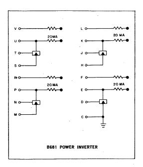
The B681 Power Inverter contains four highcurrent inverters, each with separate emitter connections. A 20-ma clamped load is permanently connected to each collector. Four additional 10-ma clamped loads are supplied. Input and output current ratings are double those of a standard inverter.
