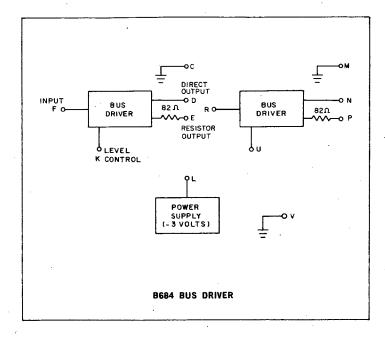
The B684 contains two dual-purpose, non-inverting bus drivers and a -3 v supply. Each bus driver provides standard levels either to a large number of inverter base and diode loads, or to a terminated 90-ohm cable. All logic terminals are available at the connector. Delay through a bus driver is approximately 30 nsec.
