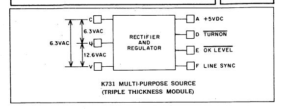
The K731 provides several specialized once-per-system control functions, in addition to operating power. Any source of center-tapped 12.6v (50 or 60 hz) allows the K731 to deliver up to 1 amp dc, which is sufficient to operate most typical control systems of up to 32 modules. This module is normally plugged into one of the innermost sockets on a K941 mounting bar, where its large components occupy space otherwise unused. The K731 is short-circuit proof.
