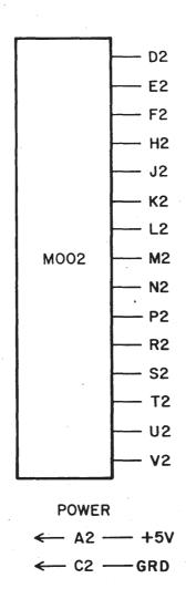
To hold unused M-Series TTL gate inputs high, the M002 provides 15 outputs at +3 volts (Logic 1), on pins D2 through V2. Up to 10 unused M-Series gate inputs may be connected to any one output. If a M002 circuit is driven by a gate, it appears as two TTL unit loads or 3.2 ma. at ground.
