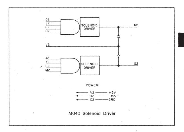
These high current drivers can drive relays, solenoids, stepping motor windings, or other similar loads. The output levels are -2 volts and a more negative voltage determined by an external power supply. One terminal of the load device should be connected to the external power source, the other to the driver output. There are two drivers per module.
