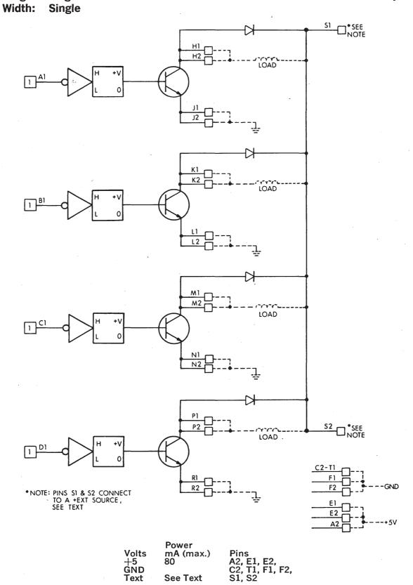
The M060 module consists of four identical high-current driver circuits. Each circuit contains an inverting gate that controls an NPN transistor switch. A low level, at any input, will turn on the switch which is capable of driving loads up to 1.2 amps with external power supply voltages of up to +75 V dc.
