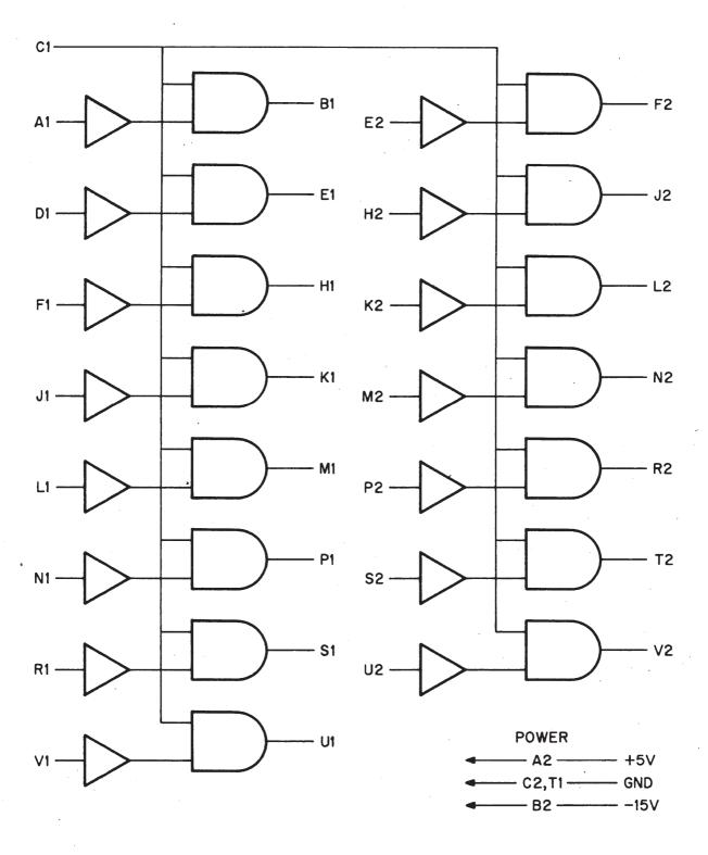
The M100 Bus Data Interface contains fifteen circuits for convenient reception of data from the PDP-8, PDP-8/I negative voltage bus. It is pin compatible with the M101 Positive Bus Data Interface.
