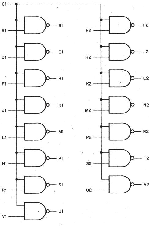
The M101 contains fifteen, two-input NAND gates arranged for convenient data strobing off of the PDP8/I or PDP8/L positive bus. One input of each gate is tied to a common line so that all data signals on the second input of each gate can be enabled simultaneously. The M101 can also be used as inverters or a data multiplexer. All data inputs are protected from a negative of more than -0.8 volts.
