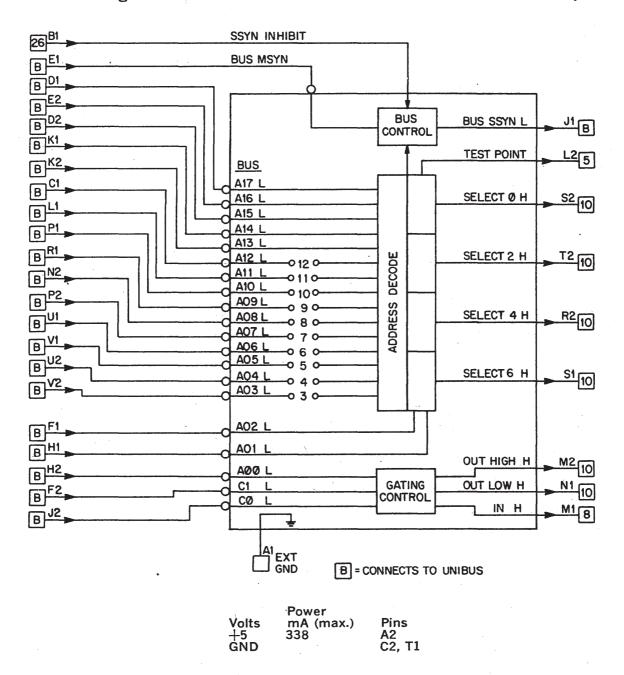
The M105 is used in PDP-11 device interfaces to control the flow of data between the device registers and the UNIBUS. It provides gating signals for up to four device registers that indicate a register is being referenced and three control signals that indicate the path for data flow.
