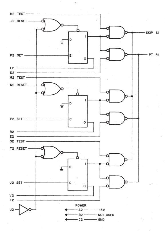
The M108 is a single height module and contains three flag flip-flops. Each flag flip-flop may be independently cleared or all flip-flops may be cleared simultaneously.
