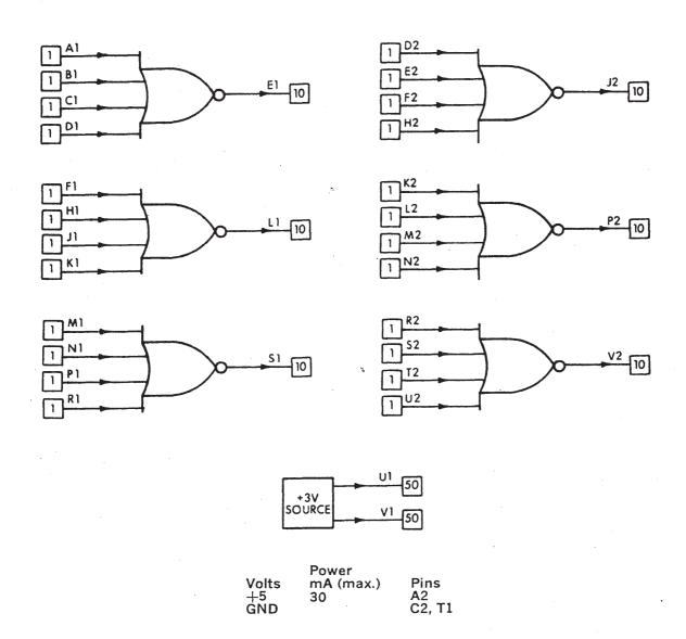
The M116 module consists of six high-speed, 4-input, positive logic NOR gates. Pins U1 and V1 provide two separate logic HIGH sources (+3V), each capable of holding up to 50 unused M Series inputs HIGH.
