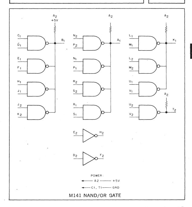
The M141 NAND/OR gate performs two levels of logic. The first is the NAND function which is identical to the M113 NAND gate. The second level is that of a wired OR for low logic levels. The two input NAND gate which is used in the M141 does not have the standard TTL output circuit, but only the lower half of the totem pole output. This allows the outputs of these gates to be connected together and to share a common pull-up resistor. Propagation delay through these gates is a maximum of 70 nsec.
