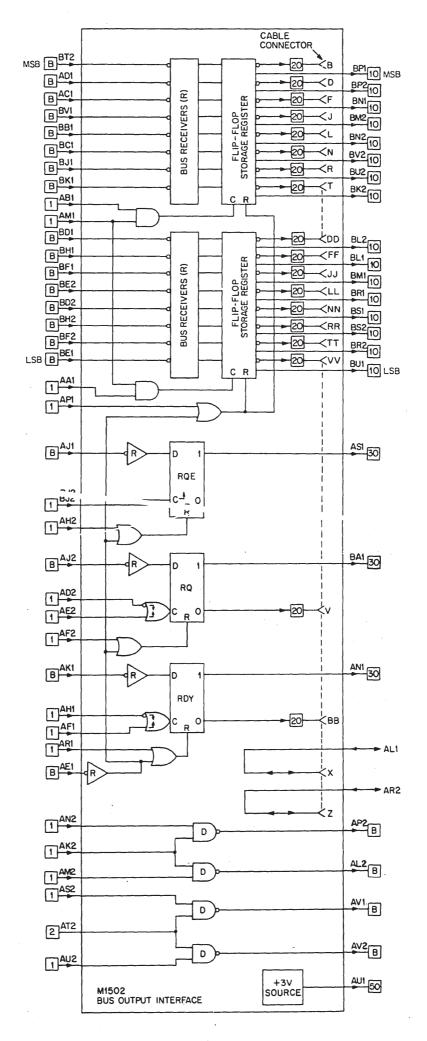
**Spare Lines:** Two additional lines are provided between the cable connector and the module for additional communication between the module and the external device. These lines are diode protected against voltage over shoot below -0.75 volts or above +5.75 volts.
