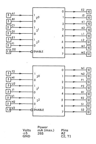
The M152 module consists of two identical binary-to-octal decoders. Each requires complementary inputs.
