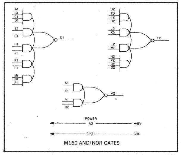
The M160 module contains three general purpose AND/NOR gates which perform functions similar to the M121. By connecting signals to the AND inputs, these gates can be used to select and place on a single output any of several input signals.
