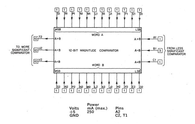
The M168 12-Bit Magnitude Comparator performs magnitude comparison of two 12-bit words. When the comparison inputs are not connected to the comparison outputs of another M168, the "A=B" input must be connected to a logical "1". The A>B and A<B inputs may individually be made a logic "1" or logic "0". However, connecting both these inputs to GND, a logic "0" is recommended.
