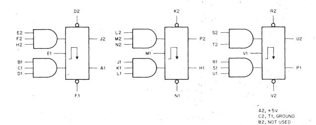
The M202 contains three J-K flip-flops augmented by multiple-input and gates. For general use as gated control flip flops or buffers.
