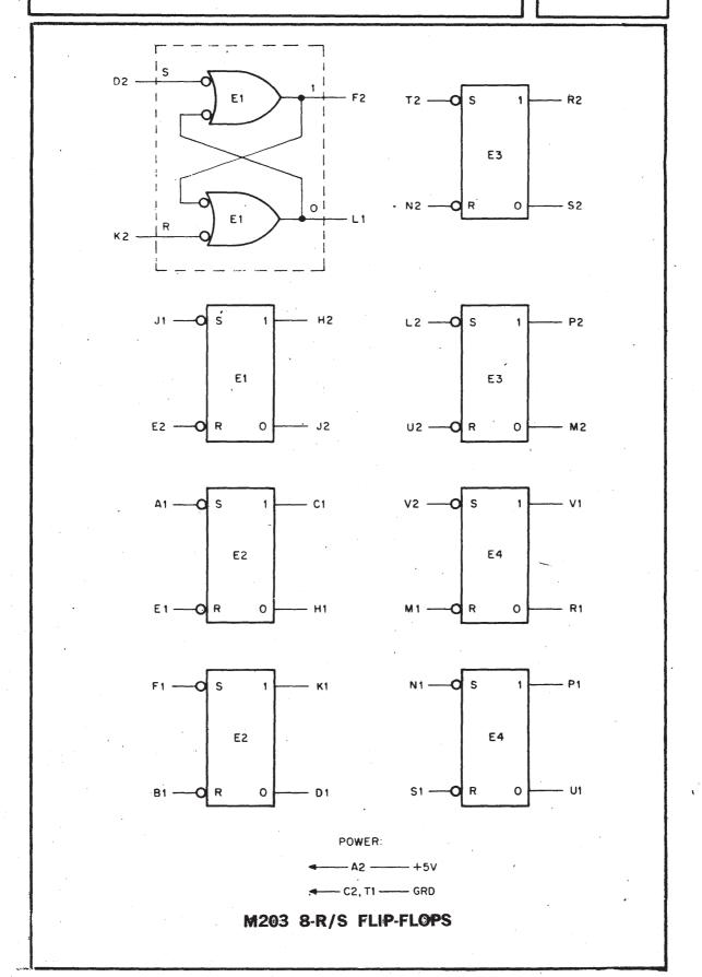
The M203 is made up of 8 R/S type flip-flops. Each flip-flop is made up of two 2-input NAND gates whose outputs are cross coupled. R/S flip-flops provide an inexpensive method of storage but care must be taken to inhibit placing the Set and Reset inputs low at the same time. In this case, the last of the inputs to be removed will control the final state of the flip-flop.
