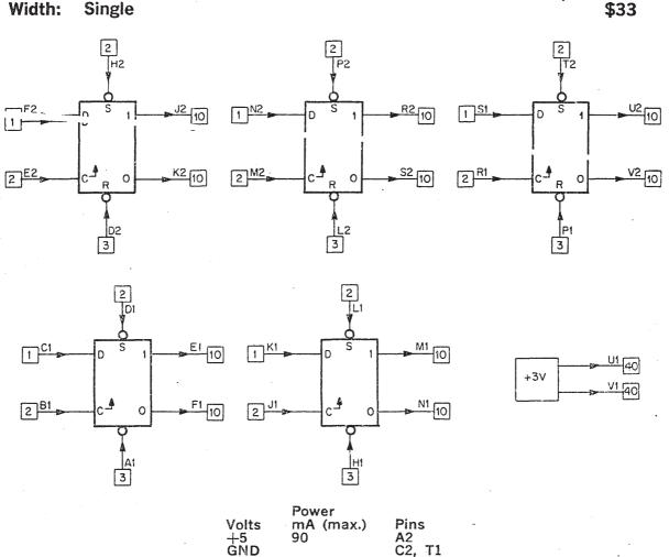
The M205 contains five separate D-Type flip-flops. Each flip-flop has independent gated data, clock, dc set, and dc reset inputs.
