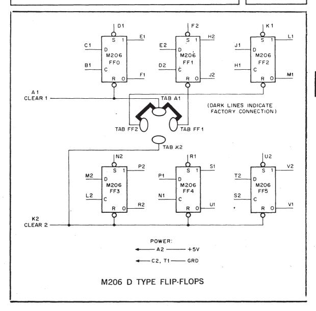
The M206 contains six separate D-Type flip-flops. Each flip-flop has independent gated data, clock, and dc set inputs.
