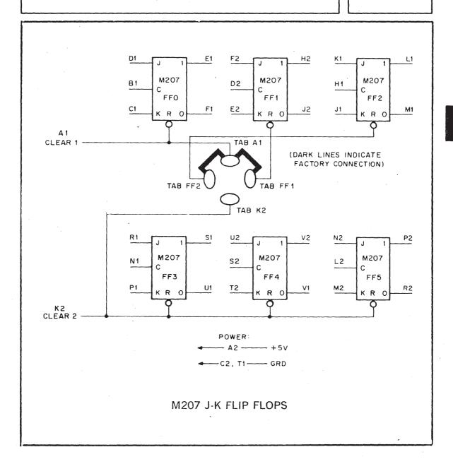
The M207 contains six J-K type flip-flops which can be used as buffers, control flip-flops, shift registers, and counters. A truth table for clocked set and reset conditions appears below. Note that when the J and K inputs are both high, the flip-flop complements on each clock pulse.
