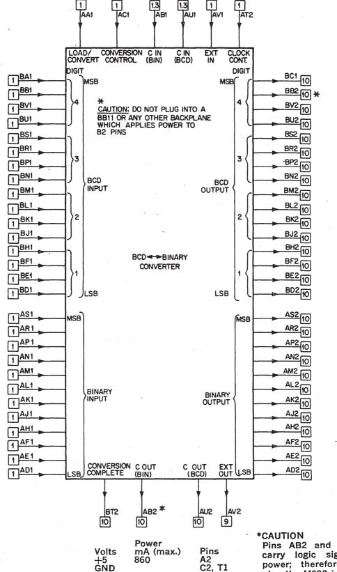
Pins AB2 and BB2 botl carry logic signals, no power; therefore do no plug the M230 into a BB1 system unit since the corresponding BB11 pins botl carry-15V.
