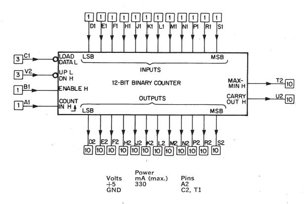
The M236 is a 12-bit synchronous binary up/down counter. It has a single control input that can switch the counting mode from up to down without disturbing the contents of the counter. The M236 is fully cascadable and programmable. Cascading simply involves paralleling the respective ENABLE, LOAD DATA, and UP/DOWN signals while one CARRY-OUT signal drives the COUNT IN input of the next M236.
