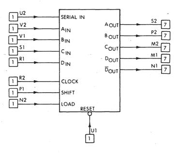
The M245 module consists of two 4-bit shift registers with both serial and parallel data entry capability. They are shift right only registers; that is, the output data is shifted from A toward D.
