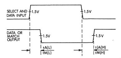
Address to data output delay  $^{t}A$  (L) = 30 ns maximum 0 ns minimum  $^{t}A$  (H) = 35 ns maximum 0 ns minimum Data bit to match output  $^{t}M$  (L) = 35 ns maximum 0 ns minimum  $^{t}M$  (H) = 40 ns maximum 0 ns minimum
