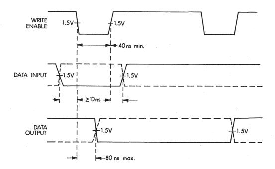
This diagram assumes that the address line is Low at least 10 nanoseconds before the WRITE ENABLE goes Low and remains Low for the remainder of the diagram.
