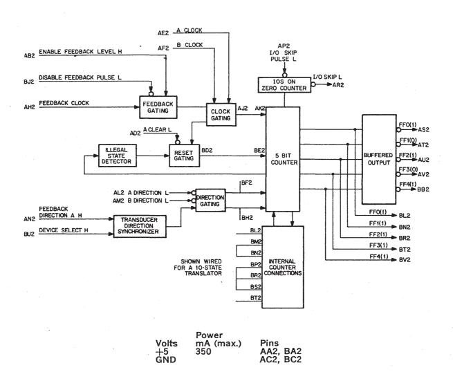
The M262 motor translator will generate the sequence of patterns necessary to step a Fujitsu type stepping motor (5 winding). It is a double height module with a five bit switch-tail ring counter which may be truncated to four or three bits by external jumpers.
