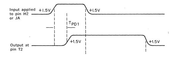
The integration period is measured from the trailing edge of the input pulse to the trailing edge of the output pulse. The approximate integration time may be calculated by the following:
