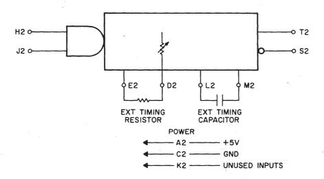
The M306 contains one integrating monostable multivibrator mounted on a single fiip-chip ™ module.
