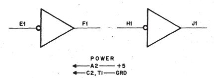
The M310 consists of a tapped delay line with associated circuitry and two pulse amplifiers. The total delay is 500 nanoseconds with taps available at 50 nanosecond intervals.
