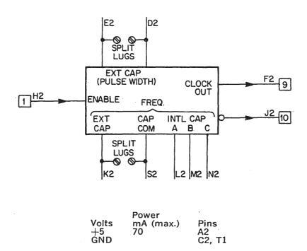
The M403 is an RC Multivibrator Clock which produces standard 10-microsecond timing pulses at repetition rates adjustable from 1 kHz to 50 kHz in three ranges. Internal capacitors, selected by jumper pin connections, provide coarse frequency control, while an internal potentiometer provides continuously variable adjustment within each range.
