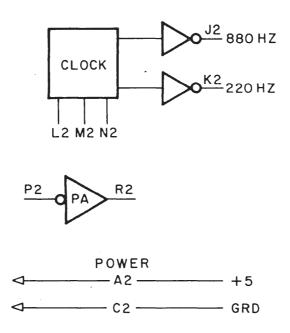
The M452 is a free running clock which generates the necessary timing signals for the PDP 8/I teletype control. Frequency adjustment of this module is limited to less than 5% and the overall clock stability with respect to supply voltage and temperature variations is about 1%. The available output frequencies are 880Hz, and 220Hz. A pulse amplifier is provided for the generation of nominal 150 nsec pulses.
