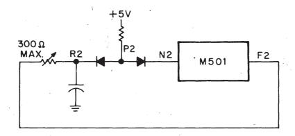
Inputs: Input signal swing on PIN R2 is limited to  $\pm 20$  volts.
