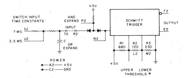
Basically a Schmitt Trigger with variable thresholds, the M501 is used as a Switch Filter, Pulse Shaper and Threshold Detector. Complementary positive logic levels are provided as outputs.
