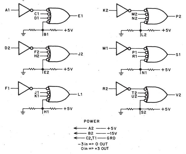
The M506 contains three non-inverting signal converters which can be used to interface the negative logic levels or pulses of duration greater than 100 nsec to M and K Series positive logic levels of +3 volts and ground. These converters operate at frequencies up to 2 MHz with typical rise and fall propagation time of respectively 70 nsec and 40 nsec.
