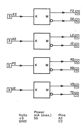
The M521 K Series to M Series Converter contains four circuits which can convert any K Series input to complementing M Series outputs.
