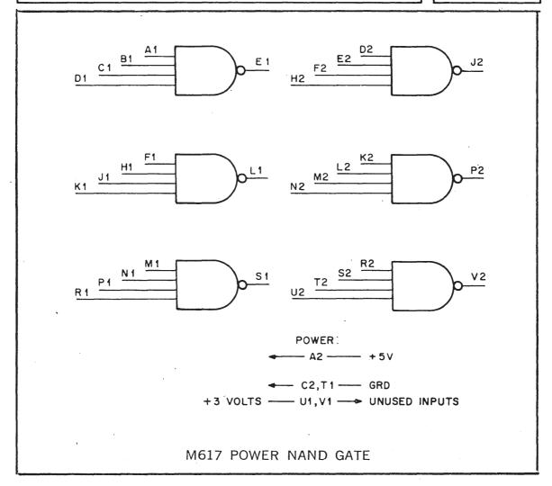
The M617 contains 6 four-input NAND gates each capable of driving up to 30 unit loads. Typical gate propagation delay is 15 nsec. Physical configuration and logical operation are identical to the M117.
